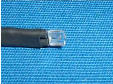
This small sensor is to be mounted inside the scanner of the copier directly to the light bar. The sensor must be located in such a way as to not be in the way of light coming through the glass. All copiers have a small section of the light bar that is hidden and out of the actual scan range. This is where the sensor must be attached. Below are several photos of mounting the sensor on a Canon iR2880i. See the captions with each photo for guidance.
